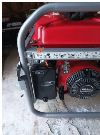
Aggregate: orange is choke and key start
