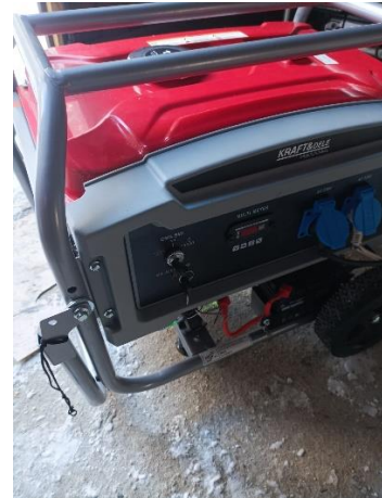
Aggregate: orange is choke and key start
